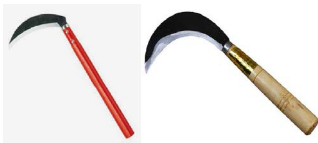
Fig. 1. Comparison of scythes between North and South China. Left: the Northern Scythe, Right: the Southern Scythe
